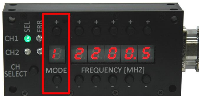
Figure 5: 2 nd Generation Switch Box Mode Selection
