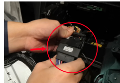
10. Take out the CarPlay 48PIN cable, plug its female side to the original car 48PIN connector.
