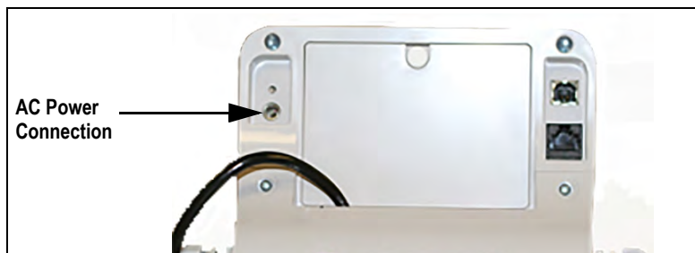
Figure 2-5. Power Connection Site
