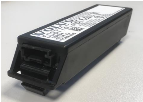
Figure: Backup Battery
