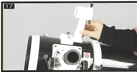
Slide finderscope base into body tube.
