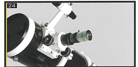
You can also use the eyepiece with 3X barlow lens, but it's hard to adjust.
