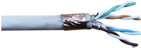
4.Fan out all four twisted pairs, following the color coding label and allocate each
