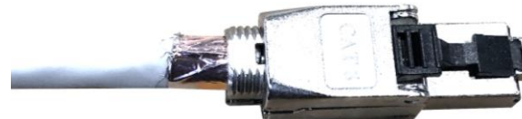
8.Close plug cover, make sure the drain wire is in proper contact with grounding clip on plug.
