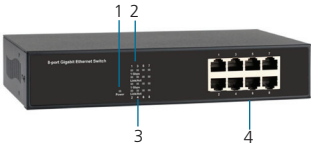
Figure 4-1. LEDs on front panel of switch.
