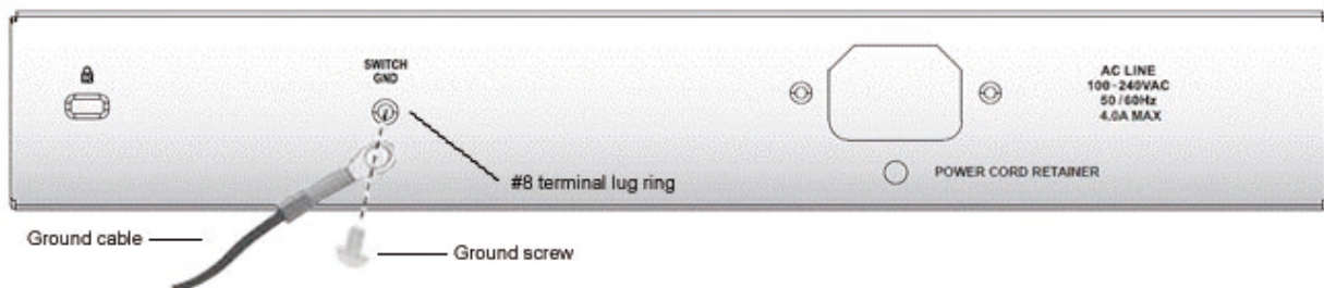
Figure 4 – Attaching a grounding cable
