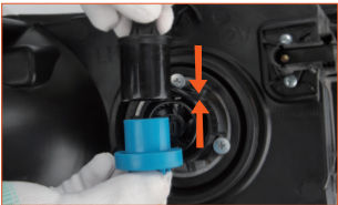
Fig. 6: Connect the power line.
