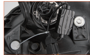
Fig. 6: Sort and fix the wiring harness with Zip Ties.
