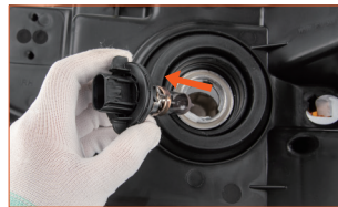
Fig. 1: Remove the OE halogen bulb
