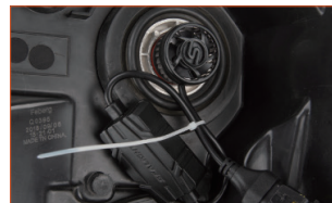
Fig. 5: Sort and fix the wiring harness with Zip Ties.
