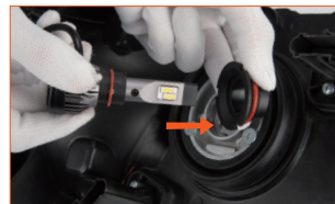
Fig. 2: Take apart the retainer holder from LED lamps.
