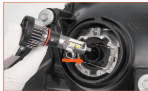
Fig. 3: Insert the lamps into the retainer holder with correct position ; Note : H4 rotate clockwise until the LED chips face 3-9 o' clock .
