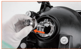
Fig. 1: Remove the dust cover and the OE Halogen bulb. and then remove the OE Halogen bulb;
