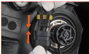
Fig. 4: Connect the power line.
