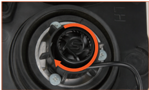
Fig. 5: Hold the base of the LED lamps, rotate clockwise until the LED chips face 3-9 o'clock. (if your highbeam and lowbeam are reverse, then rotate clockwise by 180°)
