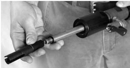
Attach coupling nut to shell cutter.
