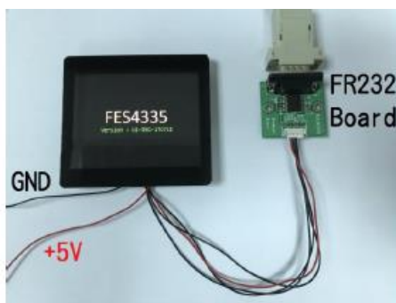
Option2. (RS232 connectivity w/ FR-DCE board)
