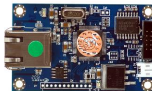
Option3. (LAN connectivity w/ FR-E2S board)
