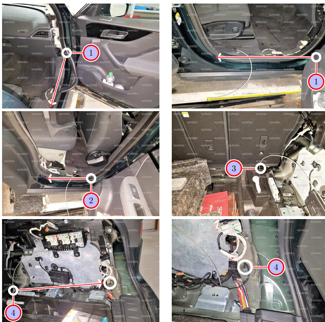
Figure 6: Cable routing to the sound generator
