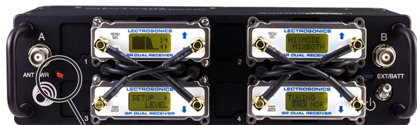
Antenna power switch glows red when DC power is enabled.
