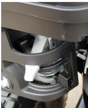
Fig4: Engine Fuel tap lever (black) and choke lever (grey)
