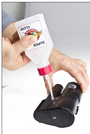
Figure 6: Suction of the excess fluid
