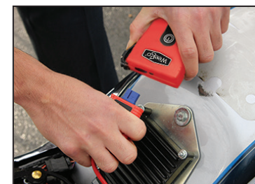
Once it Starts, Disconnect Clamps from Weego 44s
