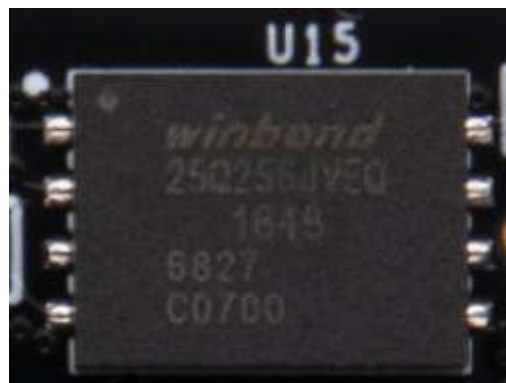
Figure 4-2 is the QSPI Flash on the core board
