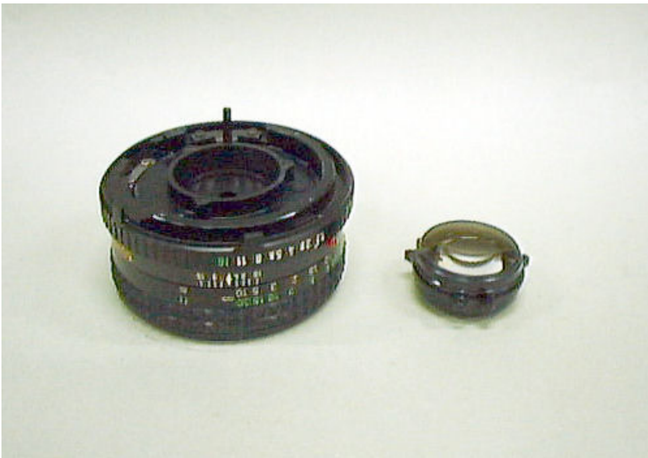
Pull out the rear lens unit.
