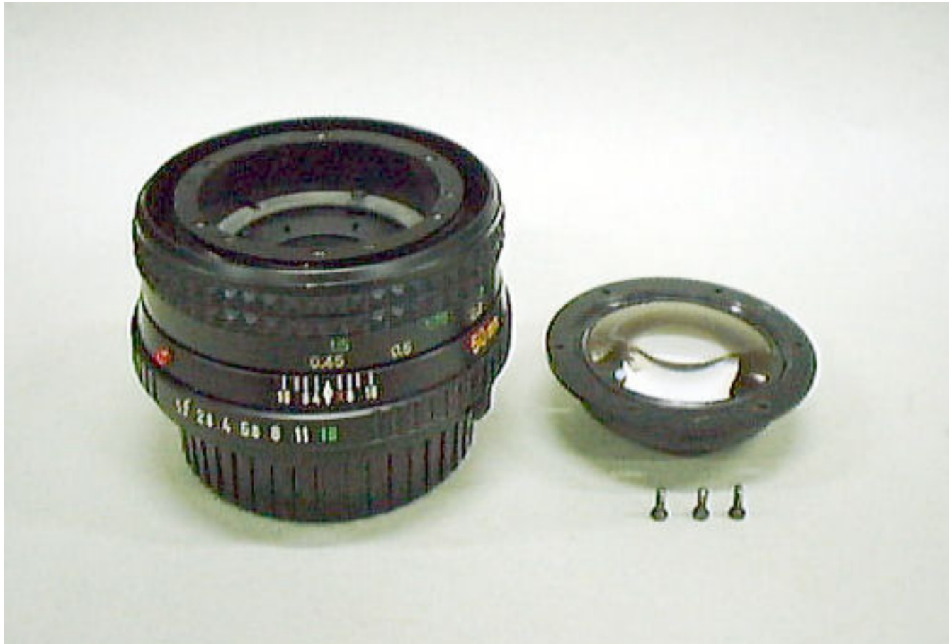
Remove the three screws to remove the filter frame cover.
