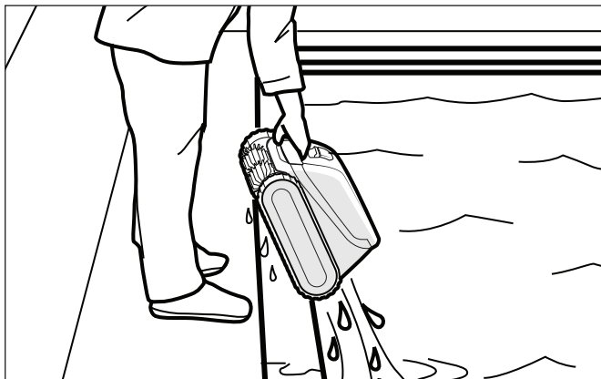
Figure 15. Keep Cleaner Vertical to Drain Water
