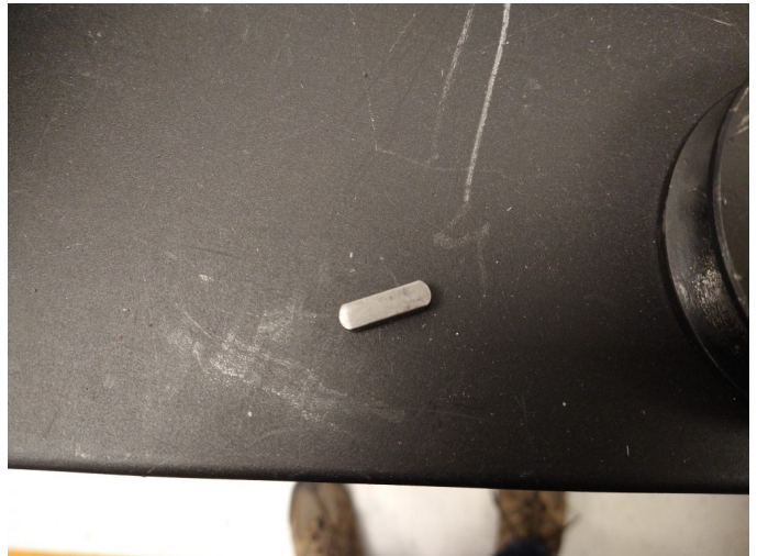
Fig. 14: Shaft key removed.
