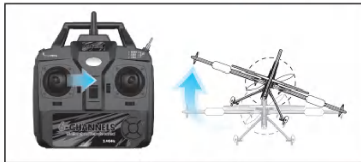
(6).右倾斜：将遥控器左操纵杆向右移动时，飞机随之向右倾斜。 Right tilt: When the left joystick of the remote control is moved to the right, the aircraft will tilt to the right.
