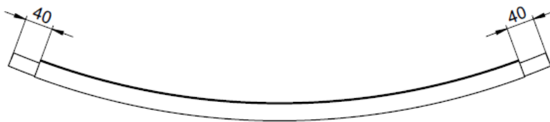
Fig. 26: Inner bend with centrally aligned insulating profile
