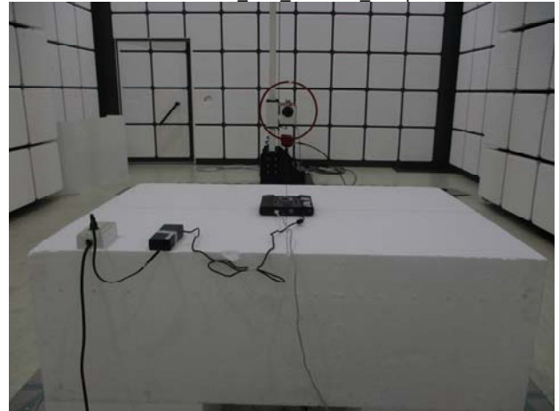
Part 15.247 BLE Radiated Setup
