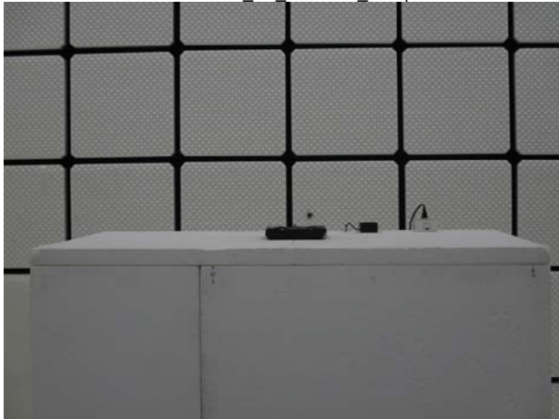
Part 15.247 BT Radiated Setup
