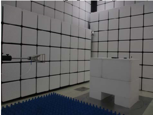
Part 15.247 BLE Radiated Setup
