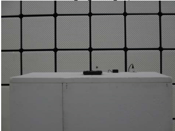
Part 15.247 BLE Radiated Setup
