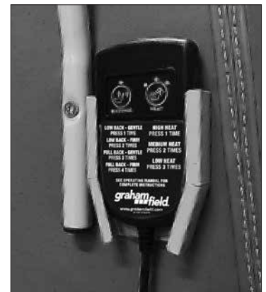
Handheld Heat and Massage Pendant Shown in Storage Bracket on Back of Recliner
