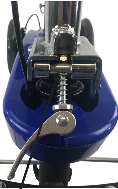
Spring loaded pin. Push to the left to release.
