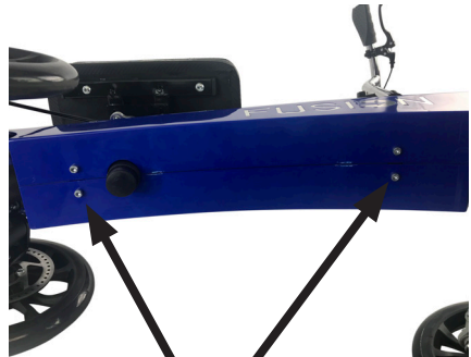
Install allen bolts with washers into the mounting.
