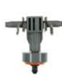
21 Inline Drip Head** pressure-regulating, self-cleaning, self-closing Art. No. 8311 2 l/h Contents: 10 pieces
