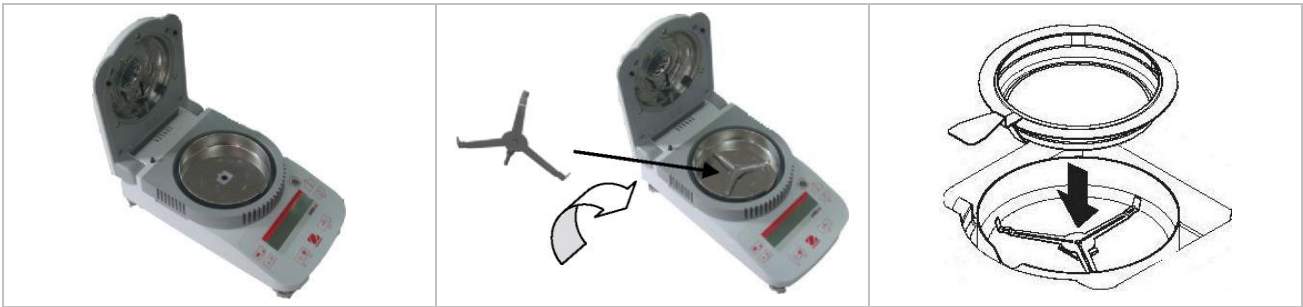
(1) Install and position Draft Shield (2) Install Pan Support, turn until it engages into position Optional Sample Pan Handler - Slide an empty sample pan under the pan handler, then place over the pan support.
