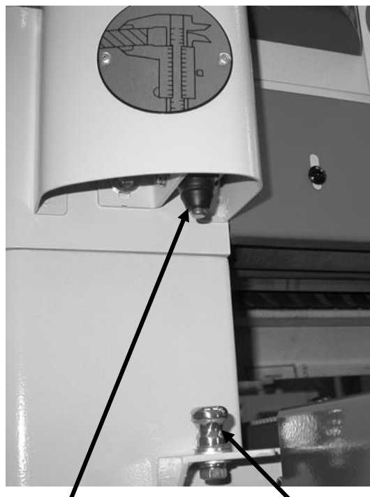
Micro switch & Height setting button
