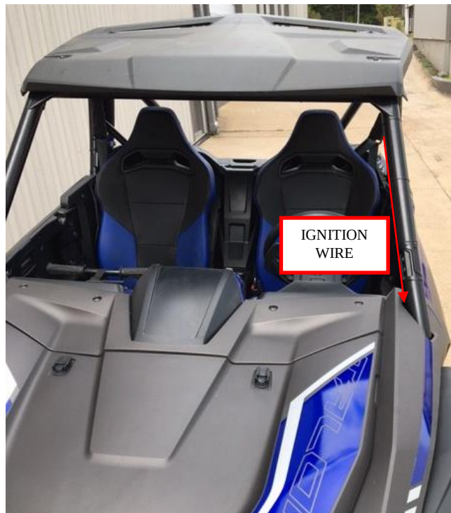
Figure 10: Ignition / connector wire routing under hood to opening.
