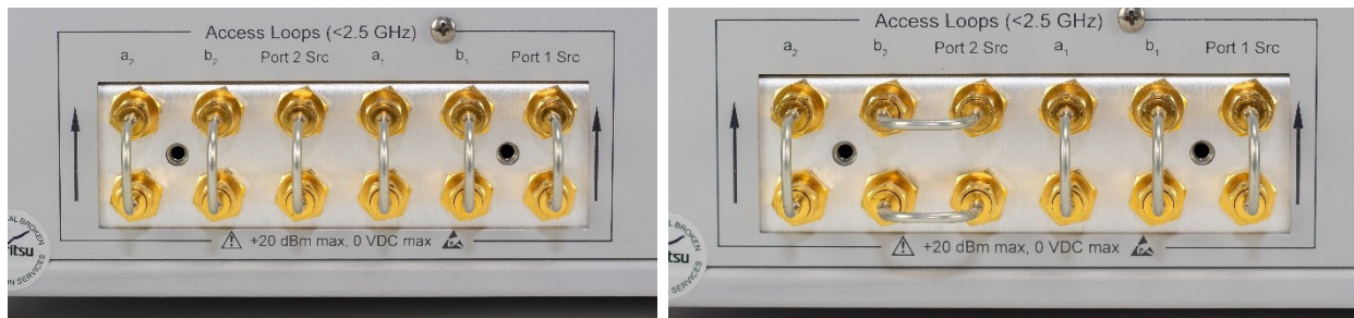
Figure 4. Rear Panel: ‘Normal’ (left) and ‘Reversed’ (right) Configurations
