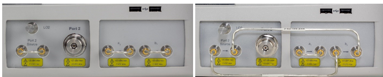
Figure 5. Front Panel: ‘Normal’ (left) and ‘Reversed’ (right) Configurations
