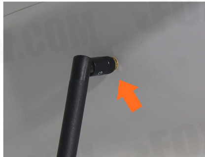
11. Install the receiver antenna.
