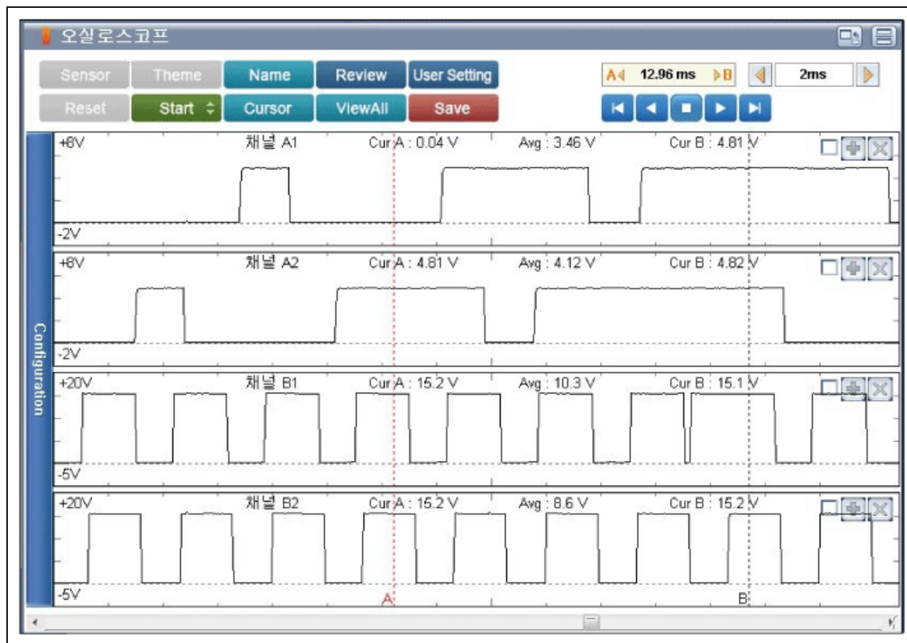
Fig 3: Screen Display - Reference Waveform During Stall Test, Duty 37% (CH A1; Intake CMPS, CH A2; Exhaust CMPS, CH B1; Intake OCV, CH B2; Exhaust OCV)
