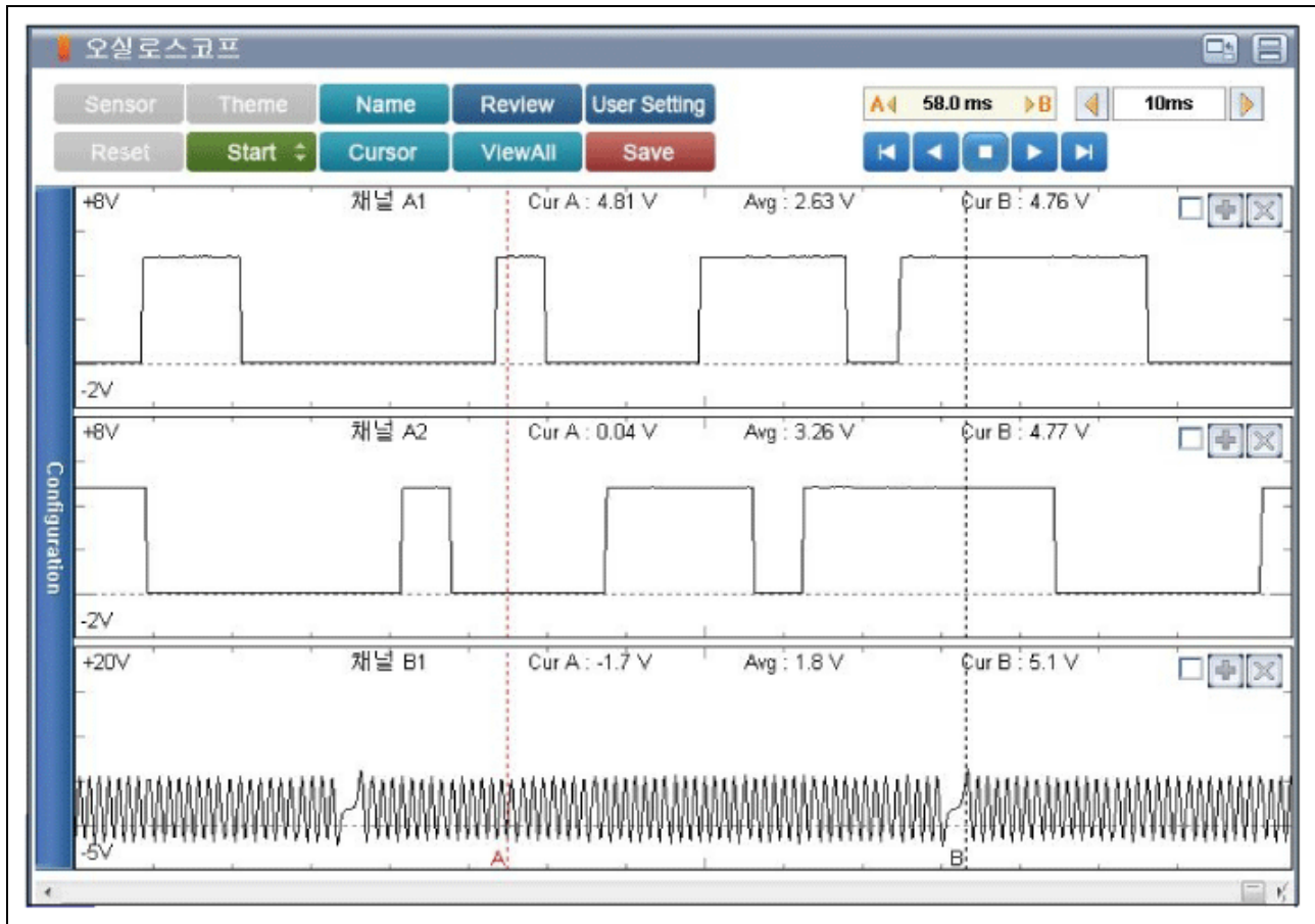
Fig 1: Screen Display - Reference Waveform At Idle (CH A1; Intake CMPS, CH A2; Exhaust CMPS, CH B1; CKPS)
