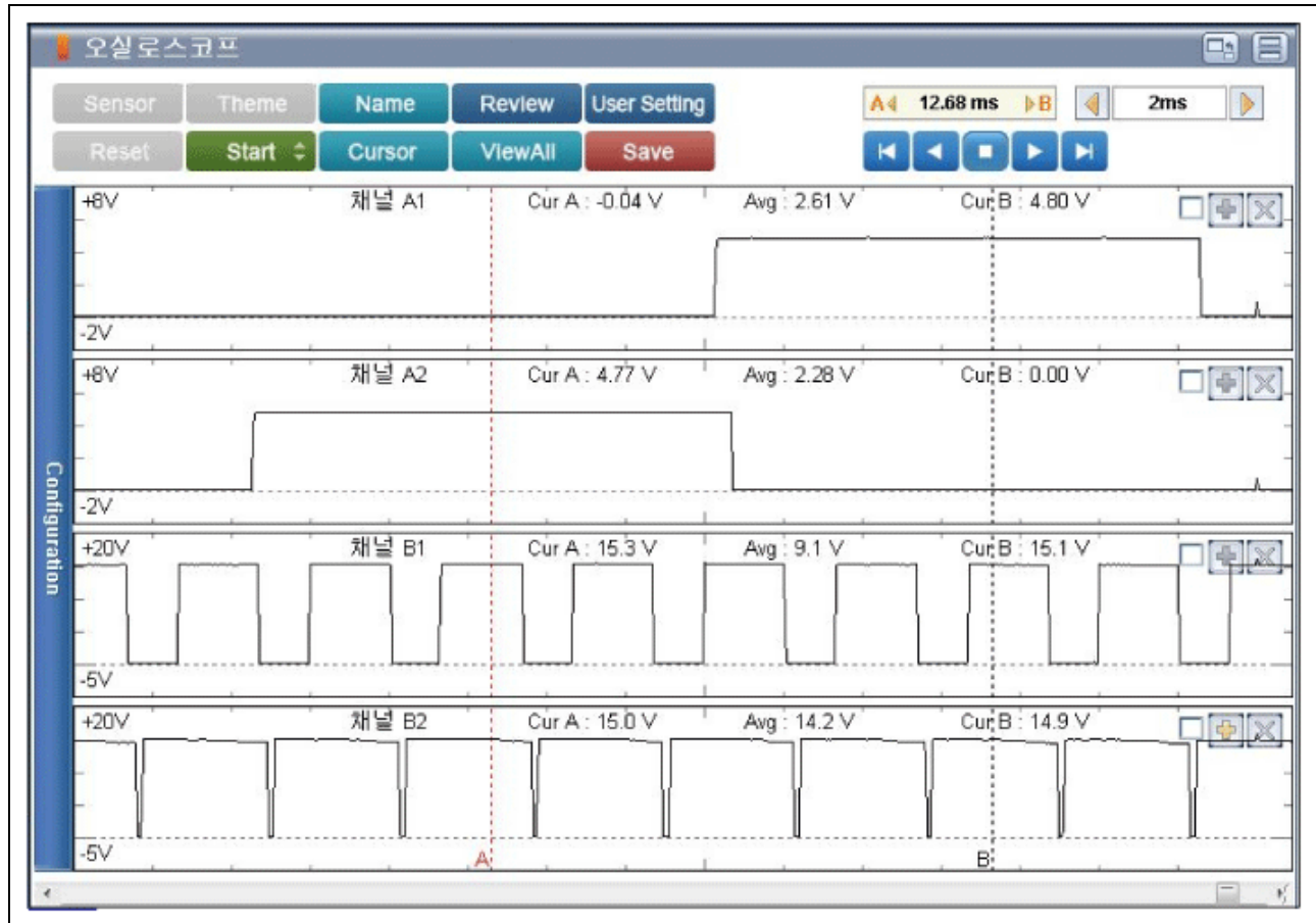
Fig 2: Screen Display - Reference Waveform At Idle, Duty 7% (CH A1; Intake CMPS, CH A2; Exhaust CMPS, CH B1; Intake OCV, CH B2; Exhaust OCV)
