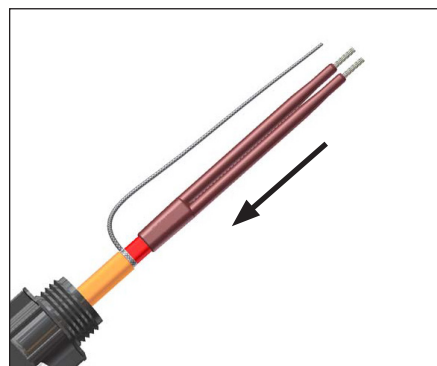
14. Slide boot onto the end of the trace heater.
