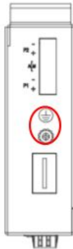
Figure 4 — The grounding screw on the switch
