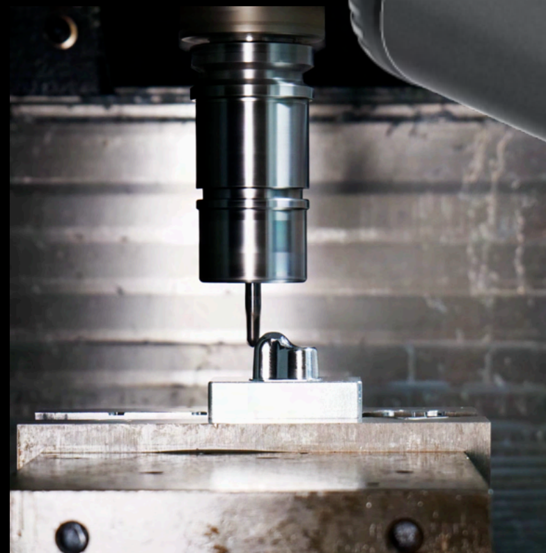
Still photograph of the CNC shell machining process.
