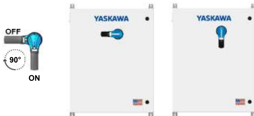
Figure 5.1 – Switch Handle Positions for OFF (left) and ON (right)
