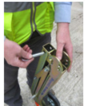
Replace locking pin on frame
