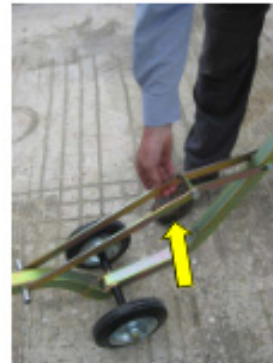
Raise front arm by lifting stay bars in front of joint
