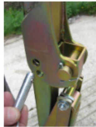
Insert locking pin (see right for alternatives)
