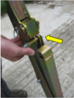
Press stay bars inwards to release front arm
