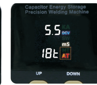
Press the 'PWR/SET' button third time to select the 'AT/ MT' two welding modes, you can switch the mode via 'UP/DOWN' buttons. Press the 'PWR/SET' button finally to save all settings and quit the adjustment.
