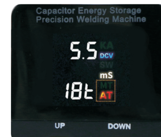
Press the 'PWR/SET' button first time to select the 'tens place' of the power grade number(the 'place' will blink once selected), you can adjust it between '0-9' via 'UP/ DOWN' two buttons.
