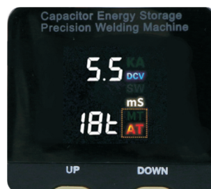
Press the 'PWR/SET' button second time to select the 'ones place' of the power grade number, in the same way, you can adjust it between '0-9' via 'UP/DOWN' buttons.
