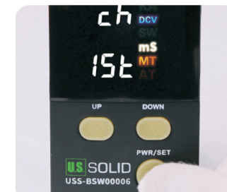
Press the 'PWR/SET' button to turn on the machine. The top half of the LED screen will display the 'CH-' signal and the actual capacitor voltage alternately and intermittently. Machine is in charging state.
