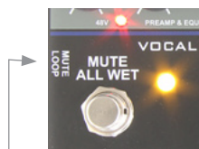
MUTE/LOOP MODE CONTROL ON SIDE PANEL
