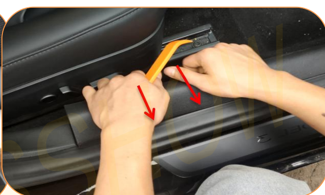
7. Remove the side cover of the passenger's footwell
