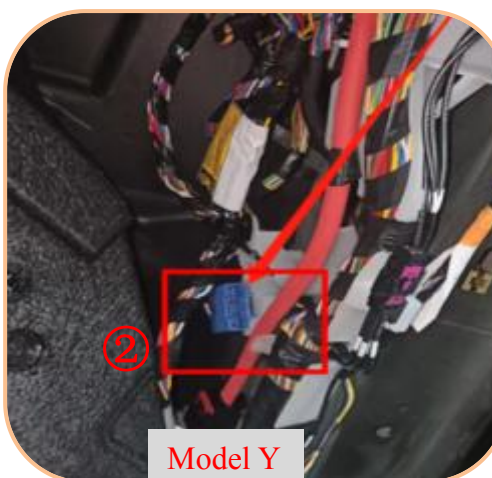
9. Connect the plug ② to the blue plug under the A pillar of the front right seat
