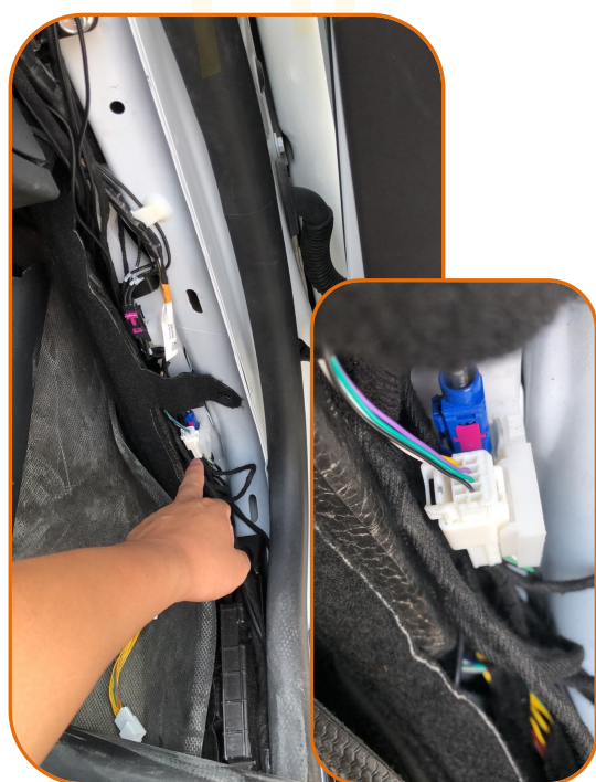
8. Connect the plug ③ to the white plug under the A pillar of the front right seat
