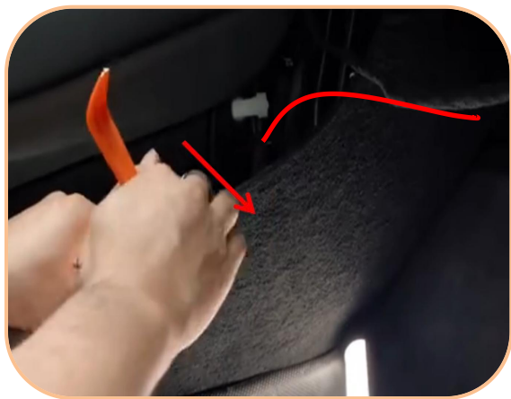
5. Pull harness ②/③ to the side of passenger's footwell
